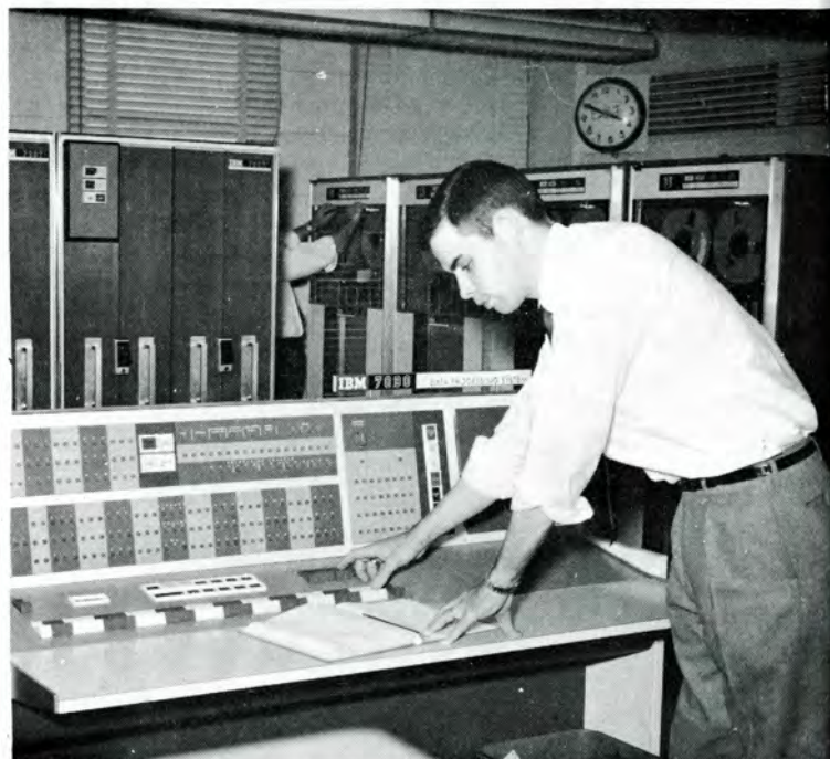
METEOROLOGIST AT THE CONSOLE OF THE IBM 7090 COMPUTER IN THE U.S. WEATHER BUREAU'S NATIONAL METEOROLOGICAL CENTER AT SUITLAND, MARYLAND, PROCESSING WEATHER DATA FOR SHORT AND LONG RANGE FORECASTS.
